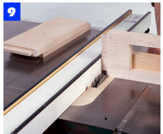
Cut the apron tenons using a dado blade in the table saw. Stand the apron on edge to cut the tenon to width.
