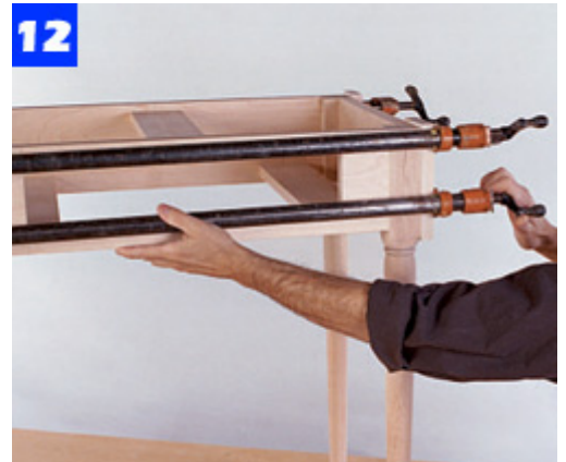
Join the legs to the apron-stretcher subassembly, then provide pressure with long pipe clamps.
