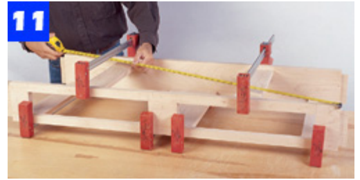
With the stretchers in place, join the rear apron to the assembly and clamp it together until the glue has set.
