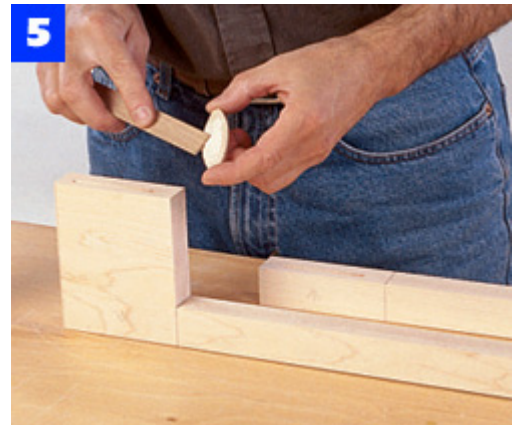
Apply glue to all the pieces in the apron assembly, including joining plate slots and the plates themselves.
