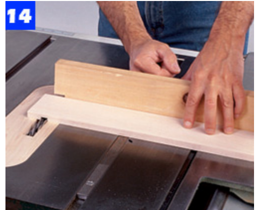
Install a dado blade in the table saw and cut the rabbets, dados and grooves in the drawer parts.
