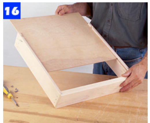
Cut the plywood drawer bottom to size, then slide it into its groove. Screw the bottom to the drawer back.
