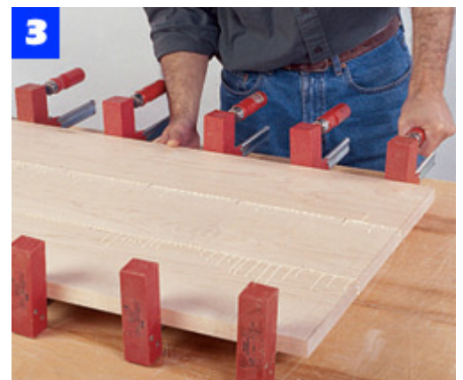
Clamp the top together until the glue has set. Use an old chisel to pare away excess glue while it is rubbery.
