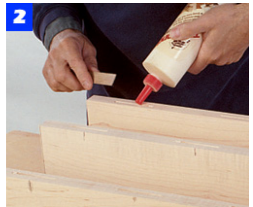
Spread glue in the plate slots, on the plates themselves and on the edges of the boards that make up the top.
