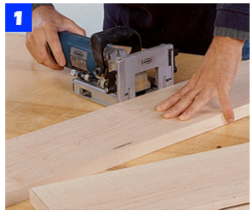
Use a plate joiner to cut the plate slots in each of the three boards that make up the
