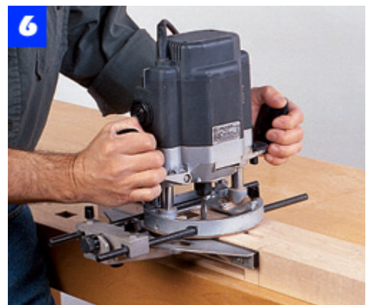
Clamp two legs together to provide additional support for the plunge router, and cut the apron mortises.
