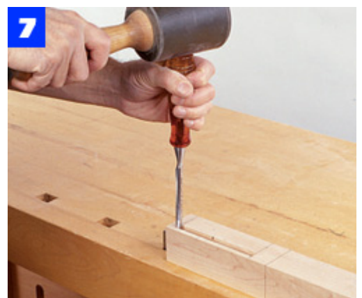
With a leg clamped firmly to the bench, chop the ends of the apron mortise square using a chisel.
