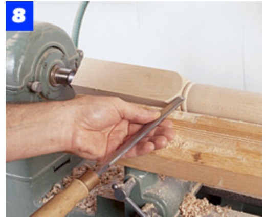
Shape the leg taper with a gouge, and then cut the bead at the leg top with a parting tool and a skew chisel.
