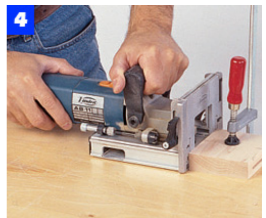
Clamp small apron blocks to the workbench in order to safely cut the joining plate slots.
